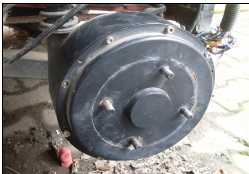
Sl. 22. Sinhroni (SMPM) pogonski motor.
